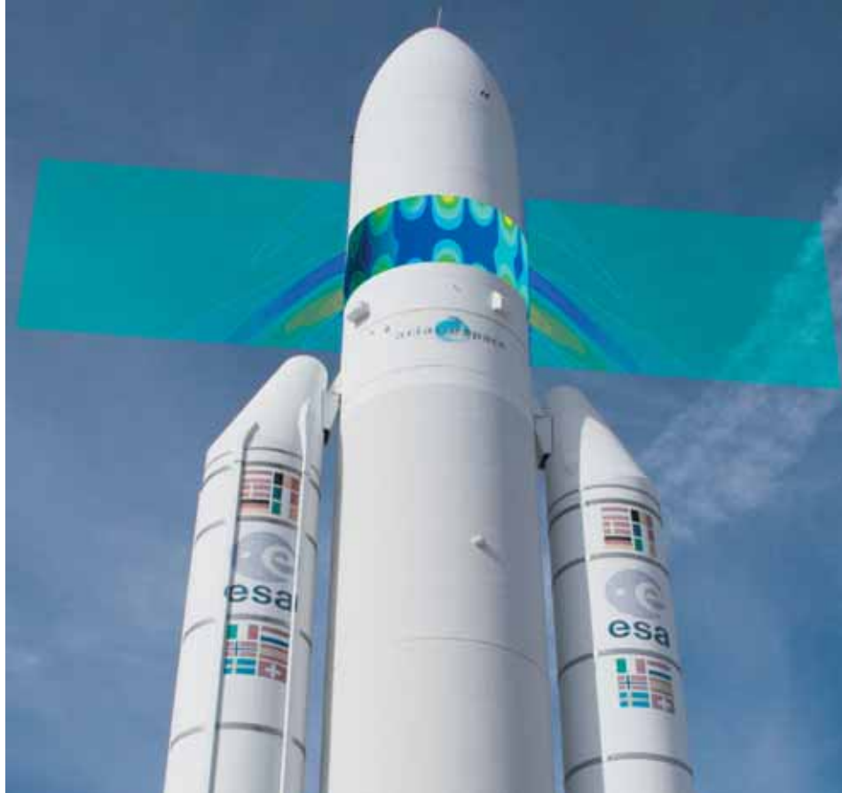
Flutter response of insulation panel during launcher ascent
