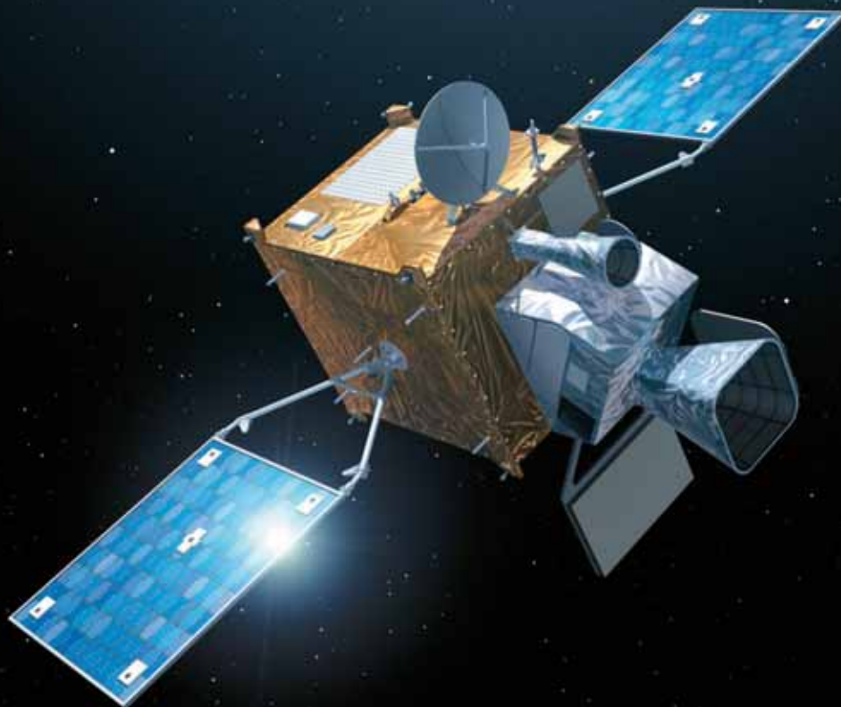
MTG – The first MTG-I Imaging Satellite is expected in 2017. Its Flexible Combined Imager (FCI) will offer advanced imaging capabilities — and ensure continuity with the current Meteosat Second Generation satellites. © ESA–P. Carril
