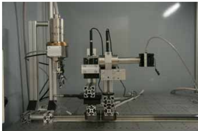
X-ray experimental facility including X-ray source (8 keV)
