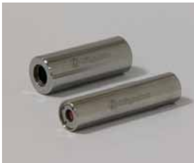
EUV elliptical optics for laboratory experiment
