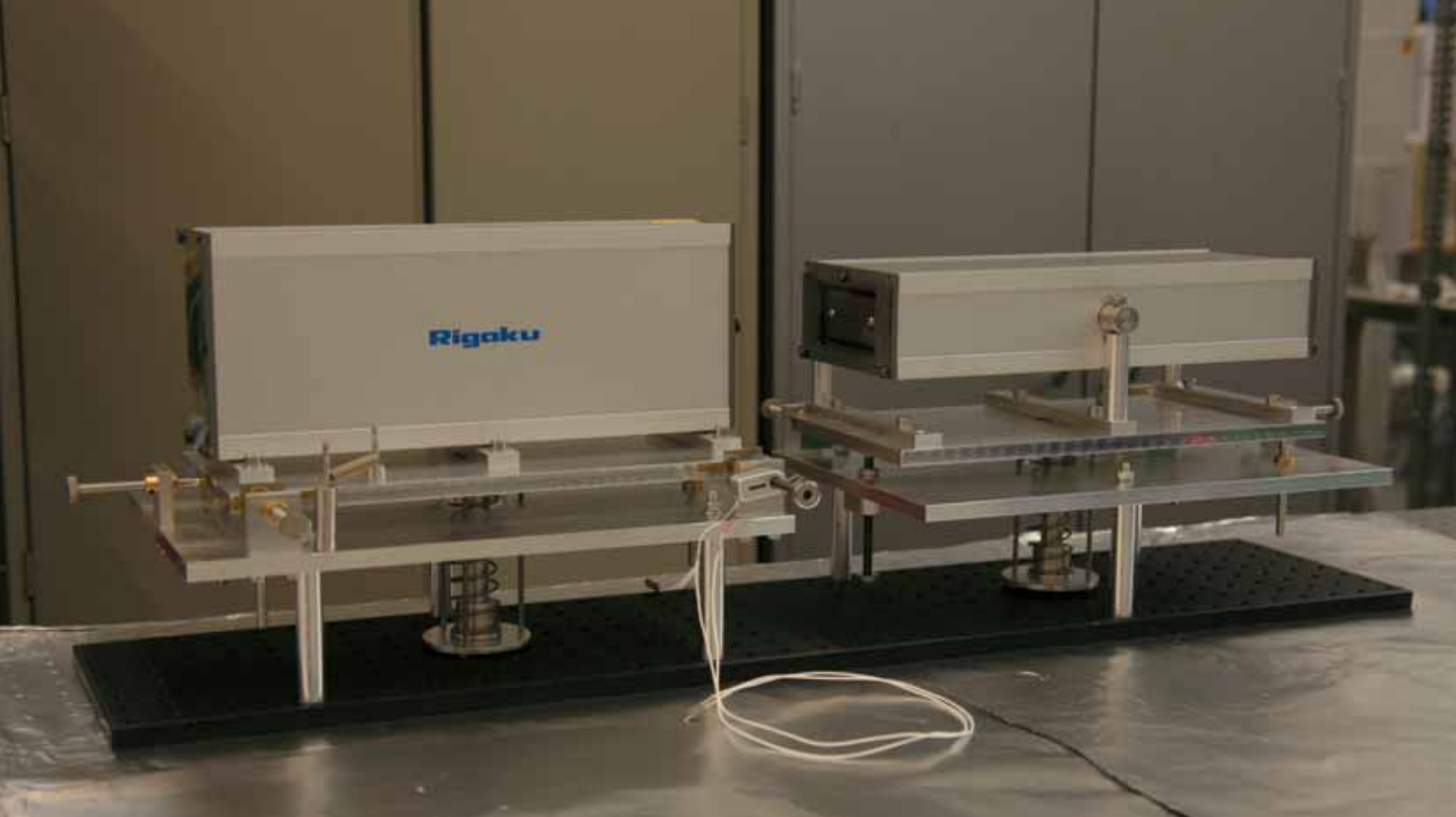
Multi-Foil elliptical X-ray optics.
